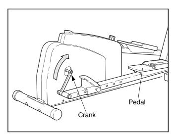
To dismount the REBEL, allow the pedals to slowly come to a stop. **CAUTION: The REBEL does not have a freewheel; the pedals will continue to move until the flywheel stops.** When the pedals are stationary, step off the highest pedal first. Then, step off the lowest pedal.
